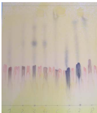
Figure 1: Chromatographic Profile of characterization of tannins in all crude extracts. Revealing- \text{FeCl}_3 (10% in \text{MeOH}/\text{H}_2\text{O} , 1:1, v/v); visualization in light of the day. Tannins are revealed as stains makes grays. 1= AdF; 2= AdT; 3= DeF; 4= DeT; 5= GIF; 6= GIR; 7= PaF; 8= PaR.
