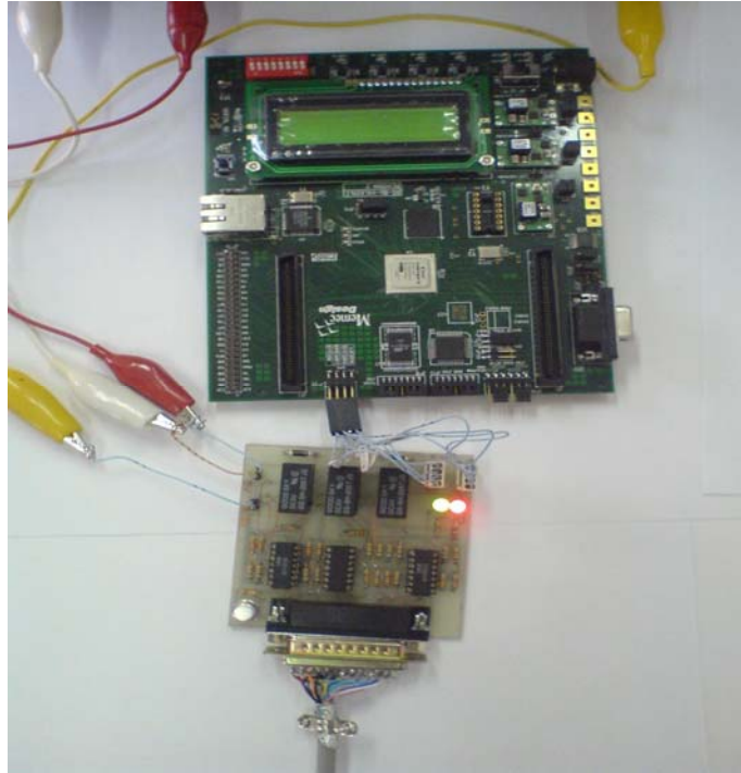
Figure 6: The FPGA evaluation board under test
